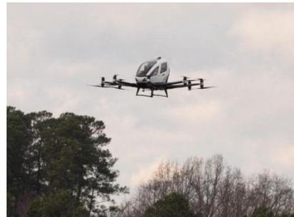
The EH 216, an autonomous aerial vehicle manufactured by EHang, flew in front of a crowd gathered at the State Highway Patrol Facility/Aviation Hangar in Raleigh. Due to Federal Aviation Administration guidelines, the demonstration flight was unmanned, but the EH 216 can carry two adults.
